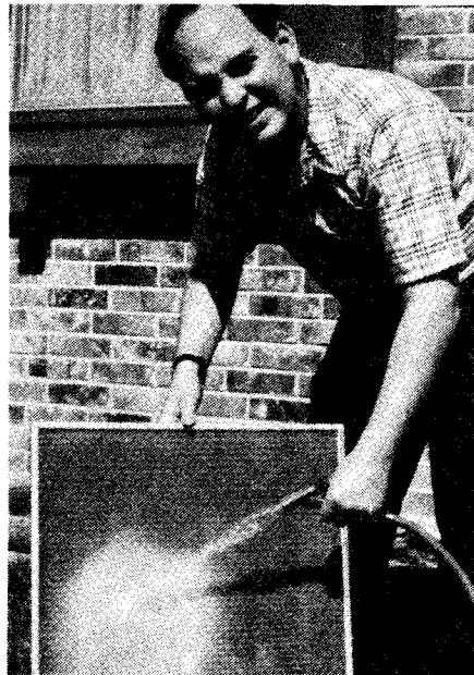
SANDY REIFLER does a quick clean job on one of his electrostatic air filters.
